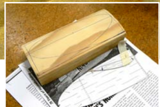
Above: A wing jig for Hornet building made by Keith Trillo.
